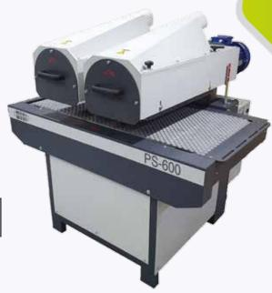
Double-spindle brushing machine PS-600 with very heavy frame as prevention from any type of vibrations during work that leads to very precise brushing or structuring effect. Open construction enables to work on work-pieces with maximum 1 200 mm width in just two passes from each side. Height of aggregates controlled electrically with maximum height of 310 mm.
